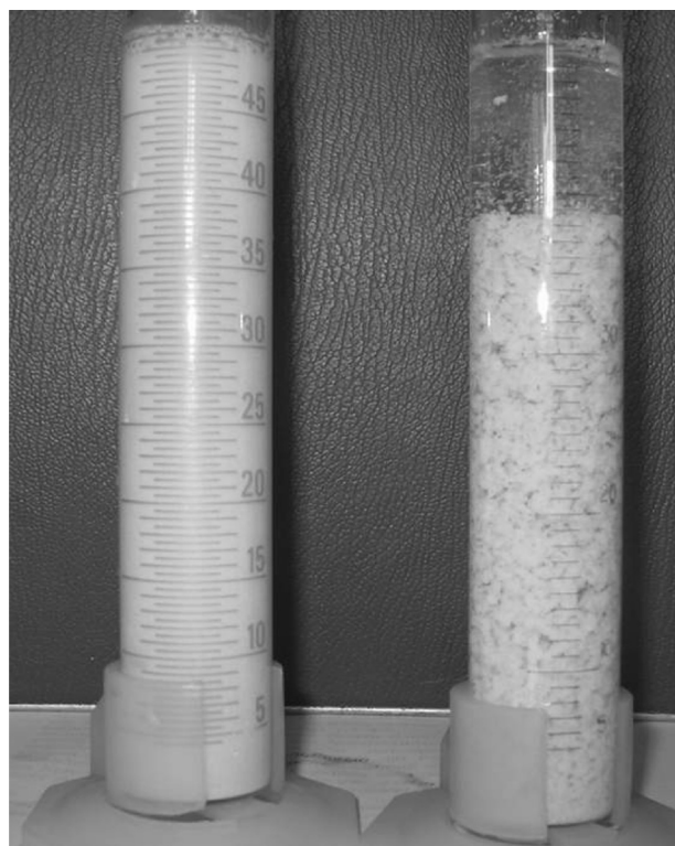
FIGURE 1 Photograph of the sedimentation cylinders in 1 min since the test beginning. Left – blank kaolin suspension; right – the suspension with the dextran-acrylamide copolymer added.
